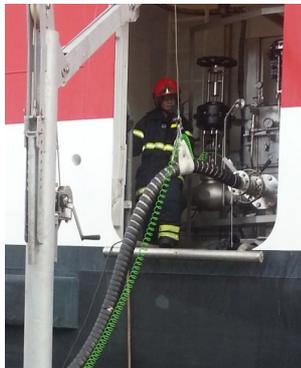
Lift the hose unit and hose into position to start the connection. Take care to support the hose end assembly so as to fit the hose unit to the tank unit in the correct orientation.
