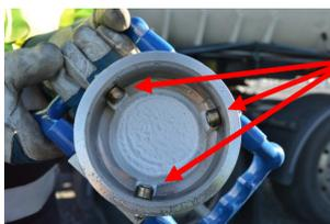
When correctly supported, the hose unit should slide easily over the tank unit. The three rollers on the hose unit engage in the three slots on the tank unit in any one of three positions at 120 degree center.
